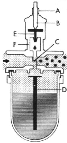
The check valve ball and spring permits the reservoir to be refilled without shutting off the air supply.
